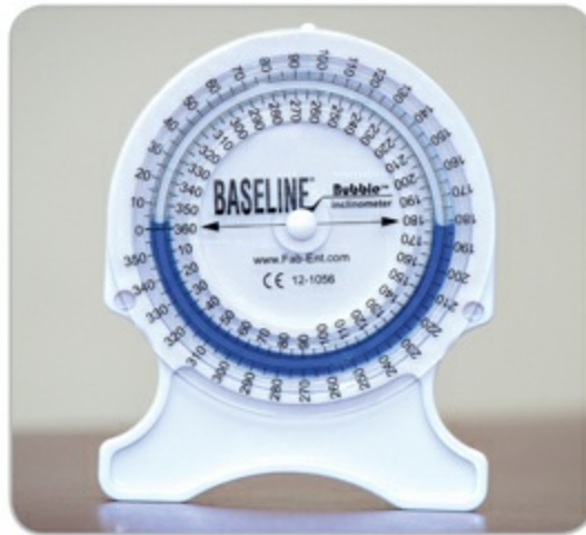
Figure 22.13. Inclinometers are fluid filled measurement instruments that use gravity's effect to measure joint position and motion. Because universal goniometers and inclinometers use different systems to measure joint motion, it is recommended that the two not be used interchangeably. (From Norkin CC, White DJ. Measurement of Joint Motion: A Guide to Goniometry . 4th ed. Philadelphia, PA: FA Davis; 2009.)
